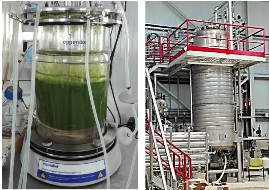
Figure 4 - A) bench 7L reactor (fermenter) producing Scenedesmus rubescens 0073 SA B) industrial 5000 L reactor. From Allmicroalgae facilities.
